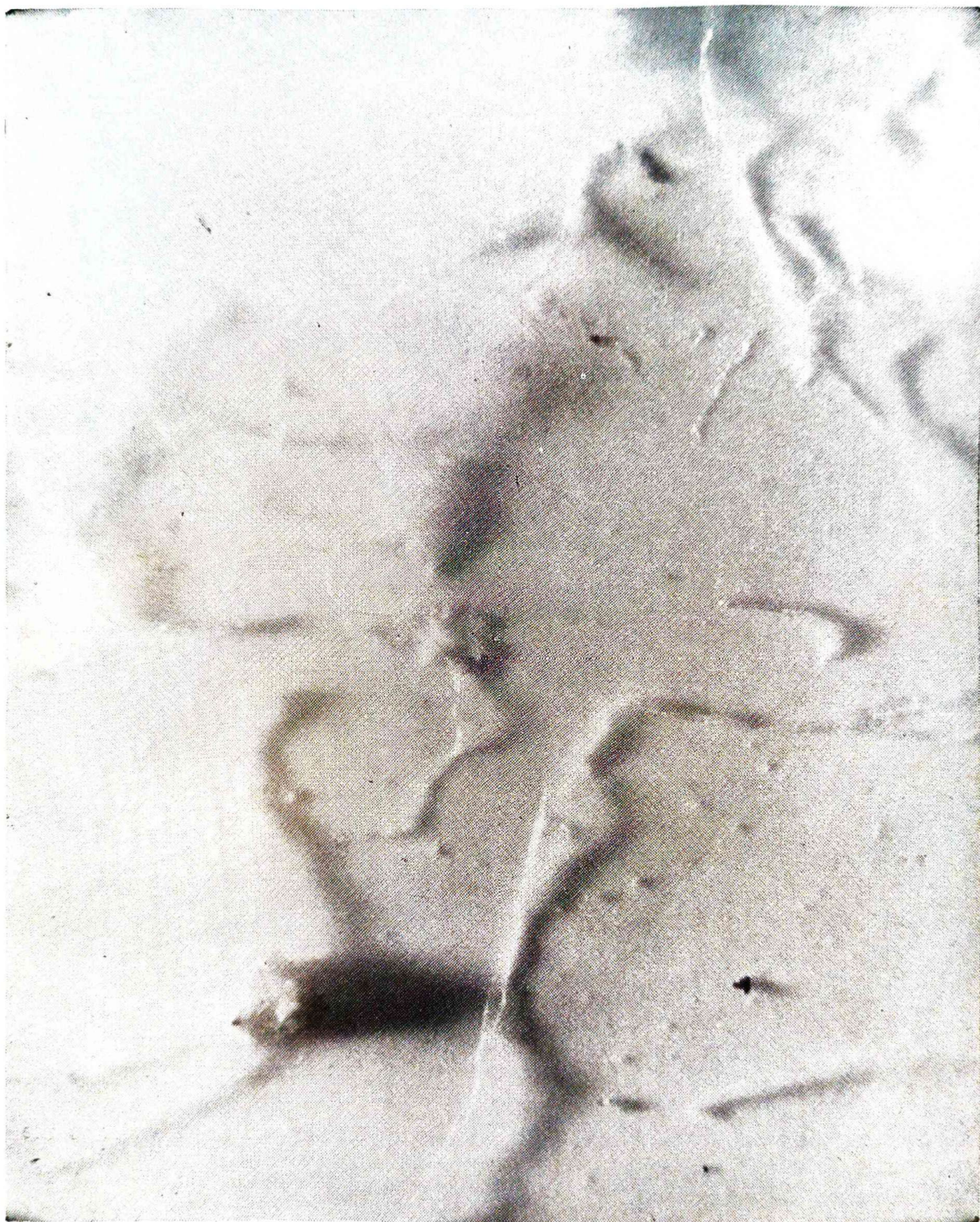
Fig. 1 — Lint and other particulate debris collected on the surface of the milipore filter from the solutions in use in an eye operating room at the end of a 30 minute procedure. The particulate matter included some metal and rubber. (Magnified about 500 times.)
